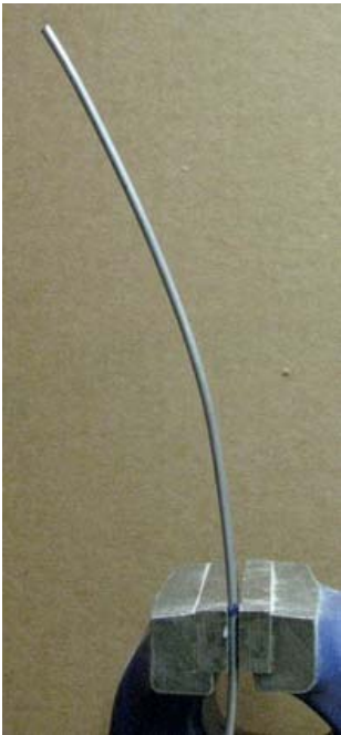
Photo 7 - Gripping the wire. The hoop is on the left and in the plane of the photo.
