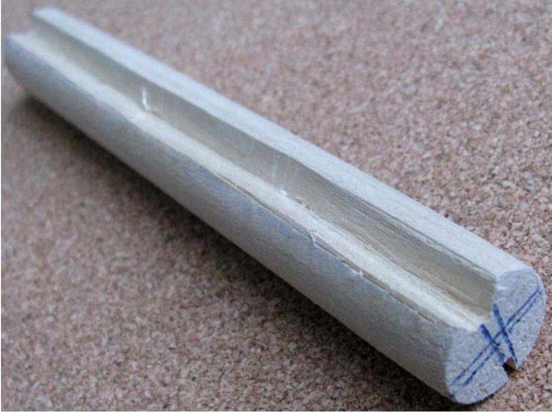
Photo 12 - The finished V-groove.
